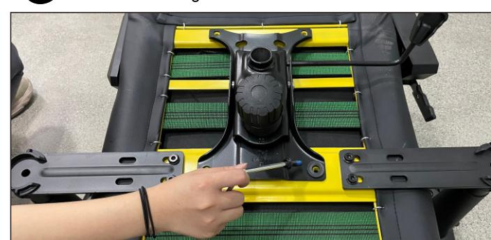
**10** Close the mechanism with side covers and fix them with M5x8 mm screws. Do not over-tight the screws to avoid damaging the plastic.
