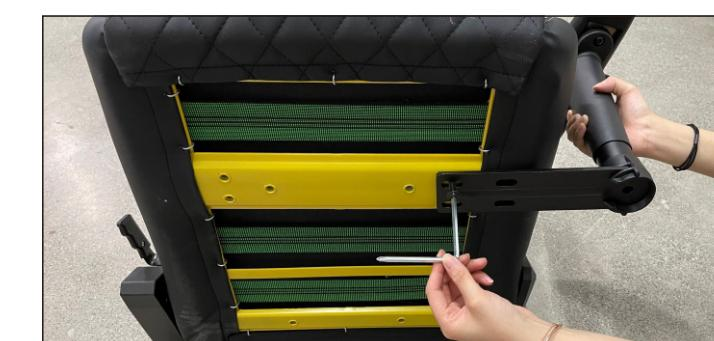
**8** Put the large washer and grover on the screw as it is shown in the picture.
