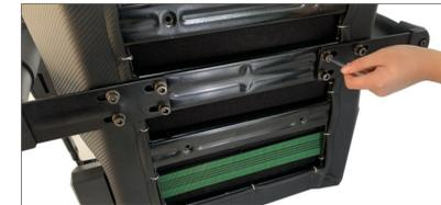
**8** Install the backrest and fix it with M8x25 mm screws. Take the screw and put grover first and then a large washer on it. Start to screw from the right hinge side, without over-tightening and avoiding distortion. Then screw the left side and after that firmly tight all the screws
